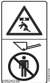
21 WARNING! Do not walk under raised lift arms. Stay a safe distance from the machine. Spare part number in USA: 15624249.
