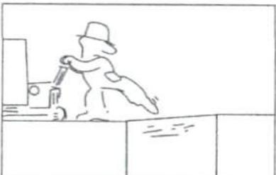
Before the truck is driven on to a loading ramp ensure that the ramp is correctly secured and has the necessary load bearing capacity. Drive slowly and carefully across the ramp keeping a safe distance to the edge.
