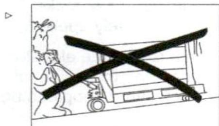
When operating on inclines the truck shall be operated with the load downwards in the direction of the incline and driven with extreme care.
