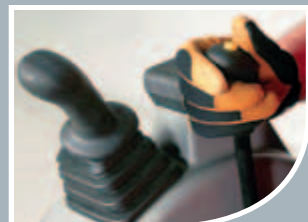
Convenient 2nd speed switch on the blade control lever.
