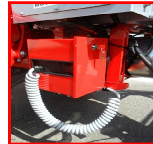
Picture 7: location for remote wired control.
