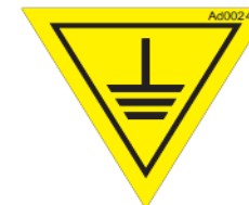
Picture 68: electric earthing.
