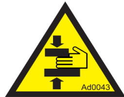
Picture 70: crushing and cutting hazard.
