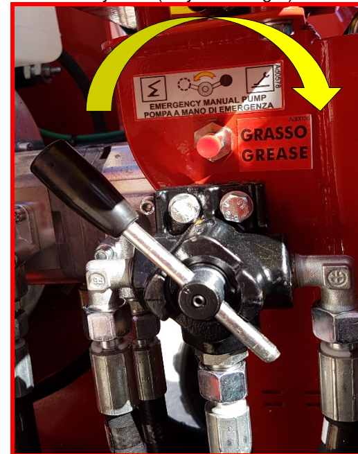
Picture 25: manual pump tap to be turned to the right.
