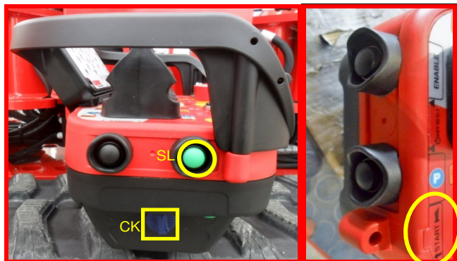
Picture 7: start/link button on radio control.
