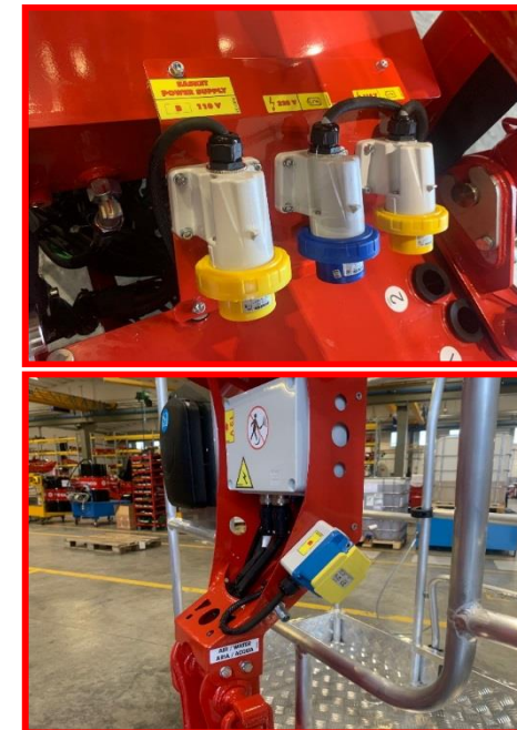
Picture 7b: dual power sockets.
