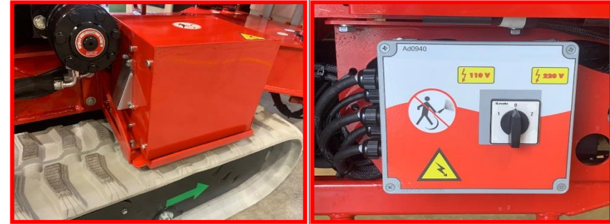
Picture 7a: alternator and selector (*optional).
