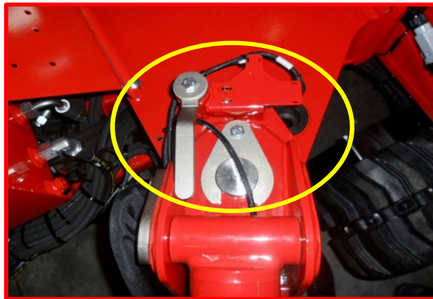
Picture 18: outrigger pins.
