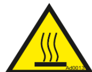
Picture 106: warning of burn risk.
