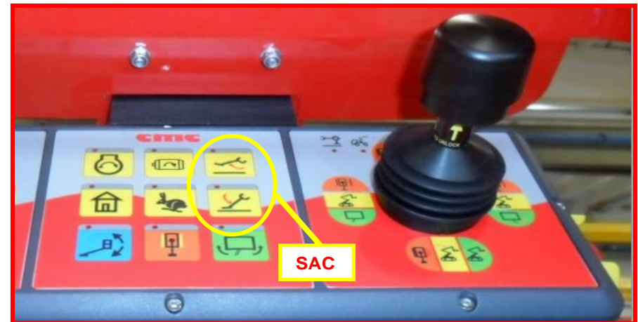
Picture 49: stabilization/destabilization lever on basket station control.
