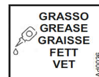
Picture 90: indication for grease application.
