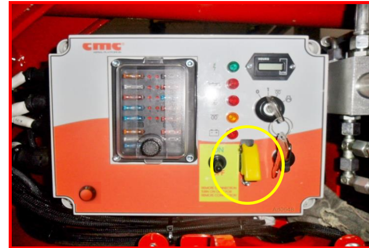
Picture 52: emergency bypass lever.
