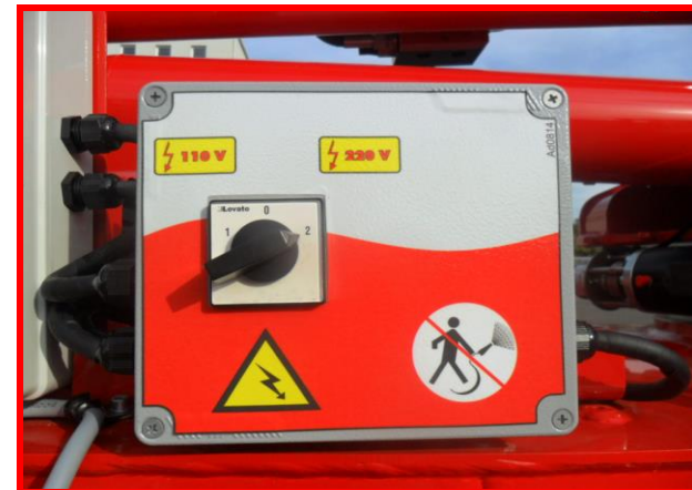
Picture 8b: transformer box with voltage selector.
