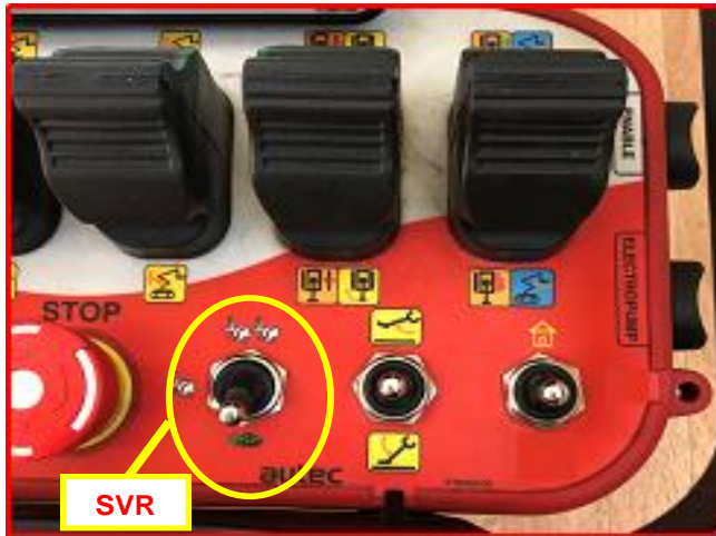
Picture 43: speed selector on travel radio control.
