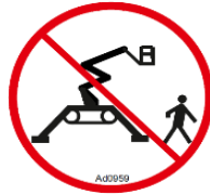
Picture 85: prohibition to stand in work area.
