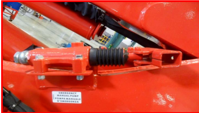
Picture 60: frame insert for manual pump.
