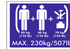
Picture 65: max capacity allowed in the basket.
