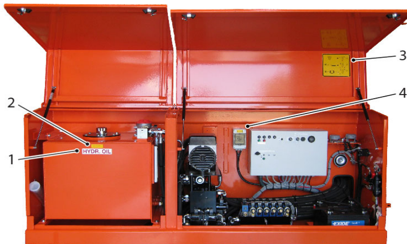
Hydraulic oil and valve/electrical compartment
