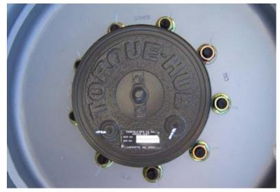
Lube Point(s) - Level/Fill Plug Capacity - 0.4 gal. (1.5 L) Lube - EPGL
