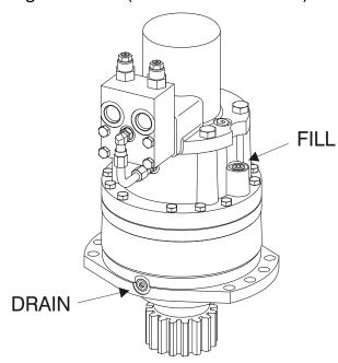
Lube Point(s) - Level/Fill Plug Capacity - 24 oz. (0.7 L) Lube - EPGL
