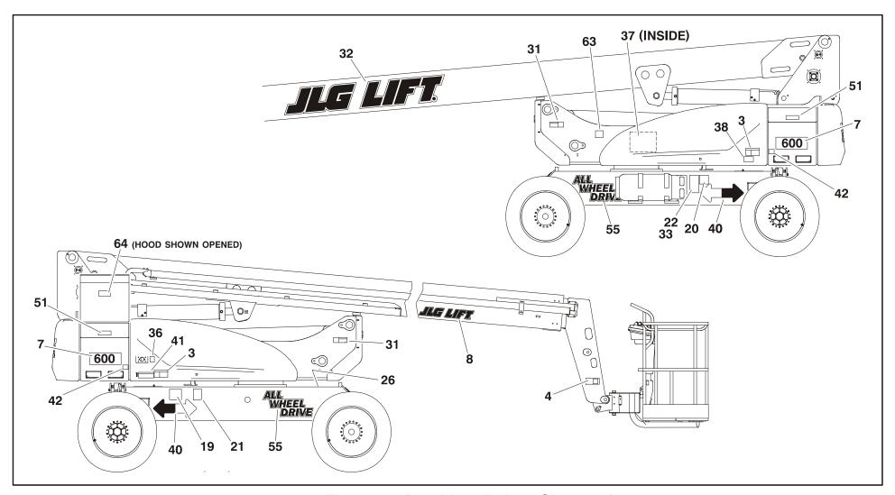
Figure 4-5. Decal Installation - Sheet 1 of 4
