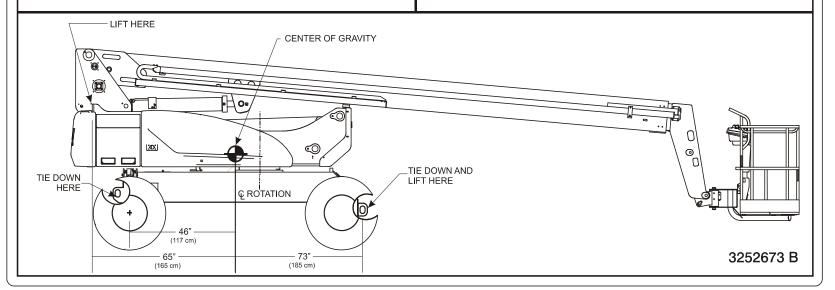
Figure 4-4. Lifting and Tie Down Chart
