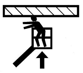
During operation, keep all body parts inside platform railing.
