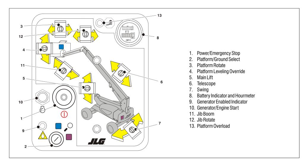
Figure 3-1. Ground Control Station
