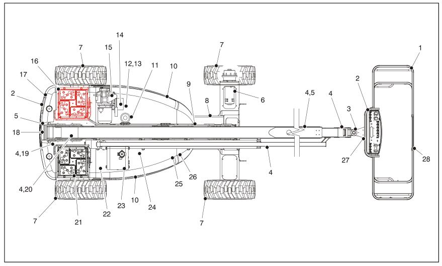
Figure 2-4. Daily Walk-Around Inspection - Sheet 1 of 4
