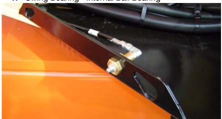
Lube Point(s) - 1 Grease Fittings Capacity - A/R Lube - MPG Interval - Every 3 months or 150 hrs of operation
