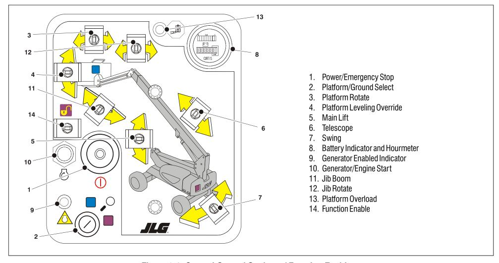
Figure 3-1. Ground Control Station w/ Function Enable
