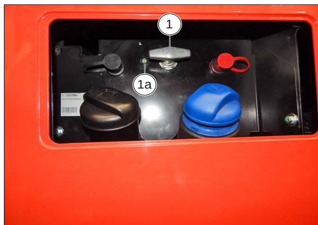
Figure 66: Battery disconnect switch
