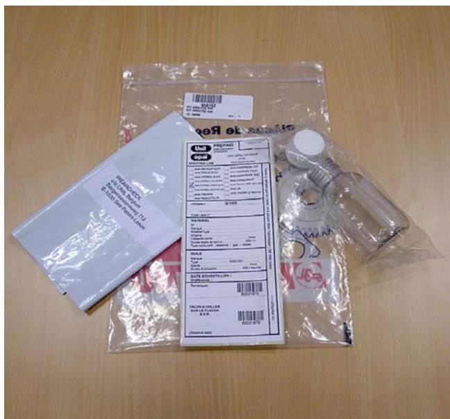
Figure 173: Hydraulic oil contamination check
