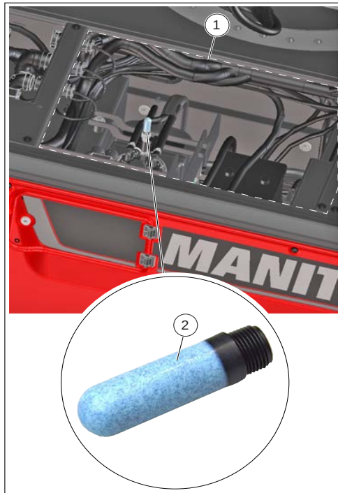
Figure 205: Replace the "DEF" tank breather
