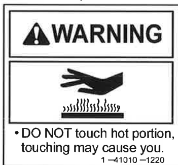
(13) Beware of high-temperature muffler (1-41010-1220)
