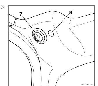
Switch the interior lighting (7) on or off using the switch (8) or button (1).
