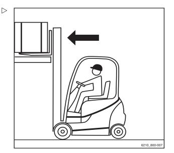
Lift the fork carriage until the load is resting entirely on the forks.
