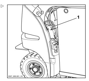
Close the battery cover completely. When doing so, ensure that no cables are crushed between the chassis and the cover.
