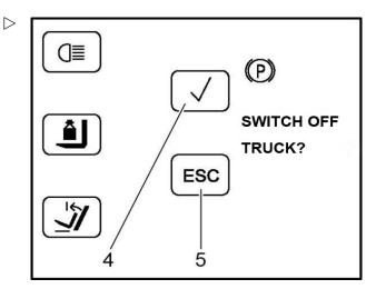
The message ARE YOU SURE? appears on the display and operating unit. To continue switching off the truck, press the soft key
