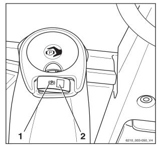
If the electric parking brake is applied, the PARKING BRAKE ACTIVE message appears in the display for 5 seconds.
