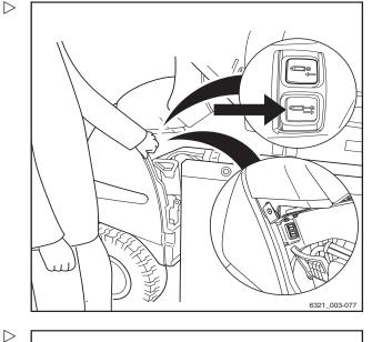
Ensure that the battery cable is not damaged when the carriage is extended.
