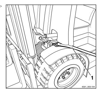
Attach lashing straps (1) to the coupling pin
