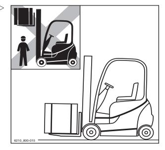
Lower the load until it rests securely on the rack.
