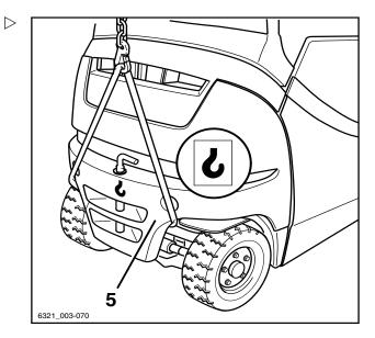
Adjust the length of the harnesses so that the lifting eye (6) is vertically above the truck's centre of gravity.
