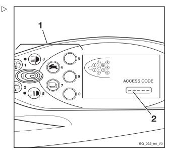
If an incorrect driver PIN is entered, the message INVALID appears for a short time. When the message goes out, the driver PIN can be re-entered.
