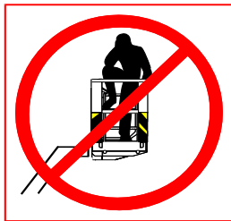
Getting in and out of the cage over the rail is prohibited!
