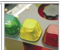
Overload warning lamps + auto stop + alarm
