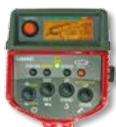
Optional radio remote control with digital feedback
