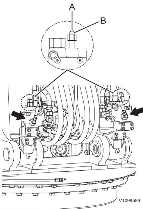
Valves rupture de flexible
