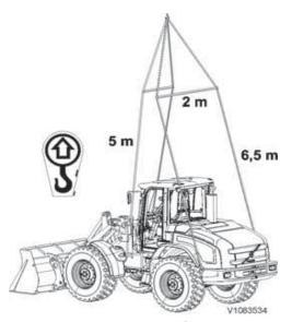
Attaching points when lifting
