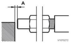
The bucket positioner is adjustable with the sensor on the tilt cylinder.
