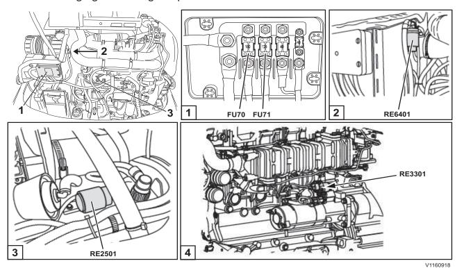
Relays and fuses in the engine compartment
