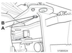
Storage position for lock bolt (A) and locking pin (B).
