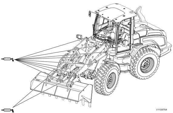
The machine may be equipped with an automatic greasing system which automatically greases many points according to a preselected lubrication cycle. The automatic greasing system should be inspected regularly and should be co-ordinated with other regular maintenance and control.
