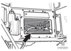
Evaporator (ventilation filters and plastic cover removed)
