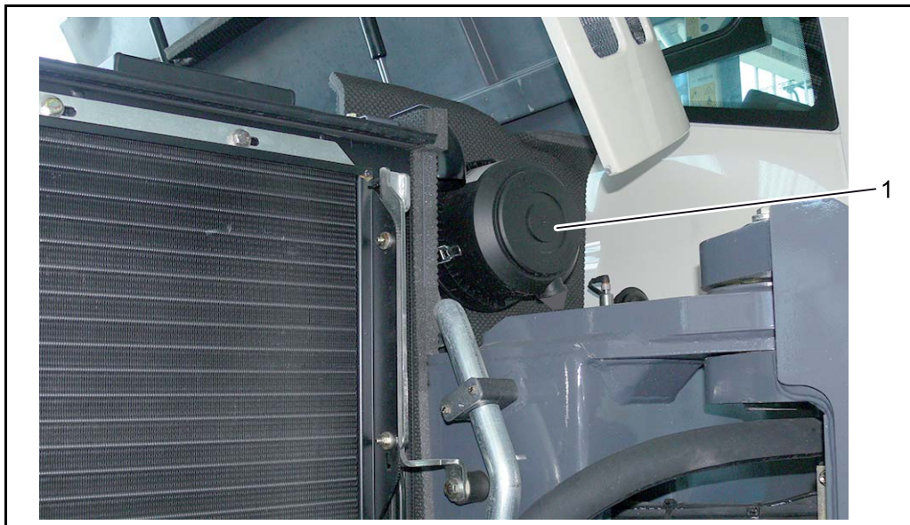
Fig. 6-9 Air filter maintenance
